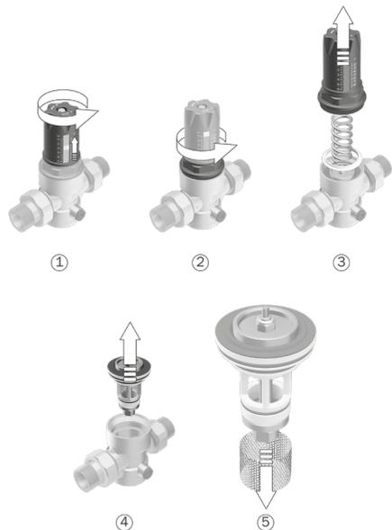
1. Close the shut-off valve placed at the inlet of the pressure reducing valve and drain the pressure for a few seconds by opening a point of use and the shut-off valve placed at the outlet; then close both.
