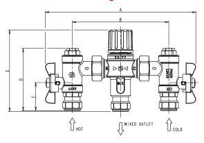
MINIMUM HOT TO MIX TEMPERATURE: 12°C **COLD WATER SUPPLY TEMPERATURE: 5-25°C HOT WATER SUPPLY TEMPERATURE: 55-65°C**
