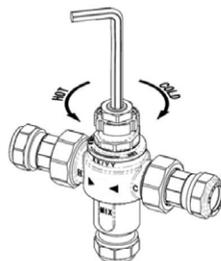
Figure 2 - D1088 pictured, temperature setting
