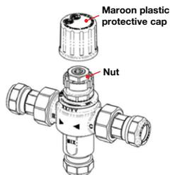
Figure 1 - D1088 pictured, cap removal
