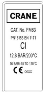
Example of Identification plates showing service pressure and temperature limitations.
