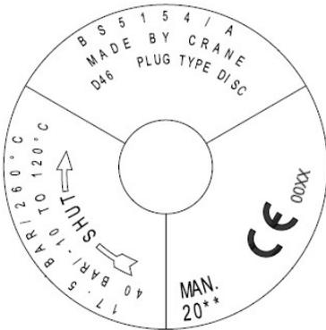
Example of Identification plate showing service pressure and temperature limitations.
